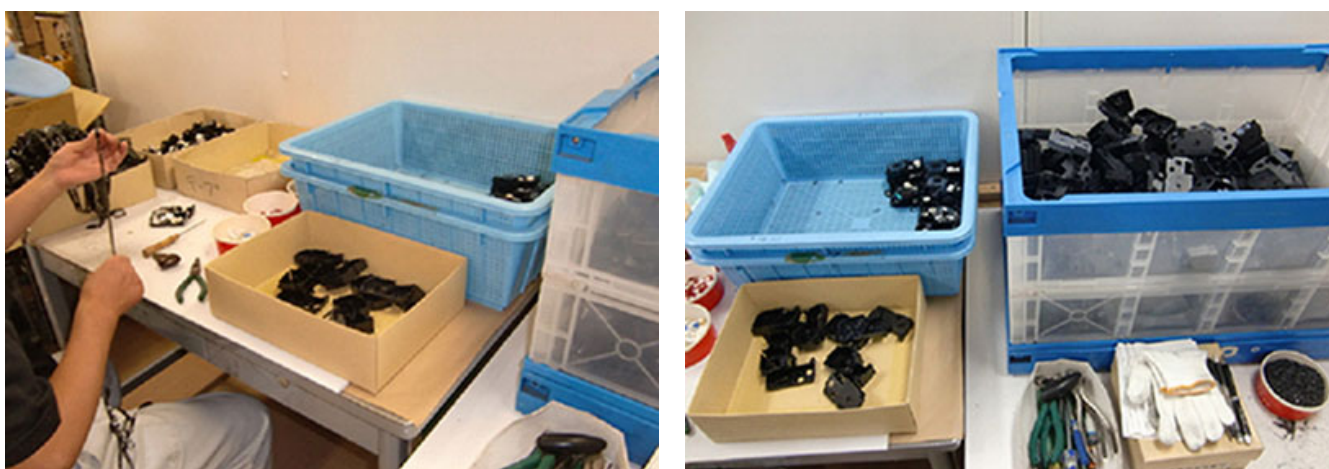
Disassembly and separation of tape cartridges and ink ribbon cassettes
